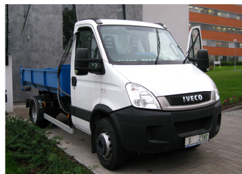
EURO 5 – DOC, DPF (particle filter), no SCR 2012 Iveco Daily, 3.0-liter Iveco engine
