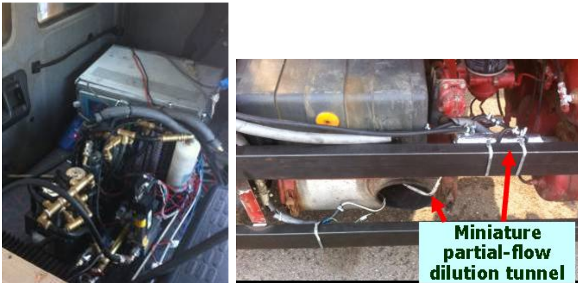
Iveco Trakker – installation of the sampling system (left, in foreground) in the cab, and of the dilution tunnel at the tailpipe (right)
