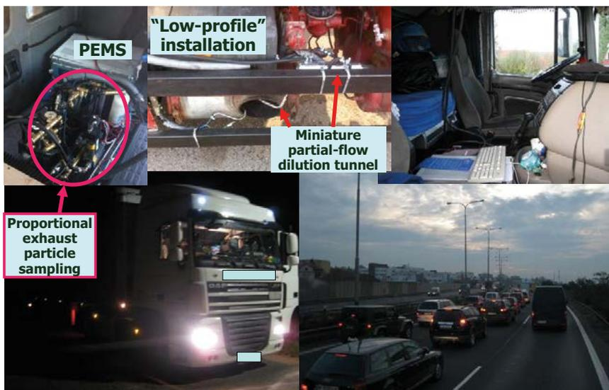
**Fig. 13: Sampling system mounted on a DAF Euro 5 truck with a SCR NO<sub>x</sub> reduction catalyst.**
