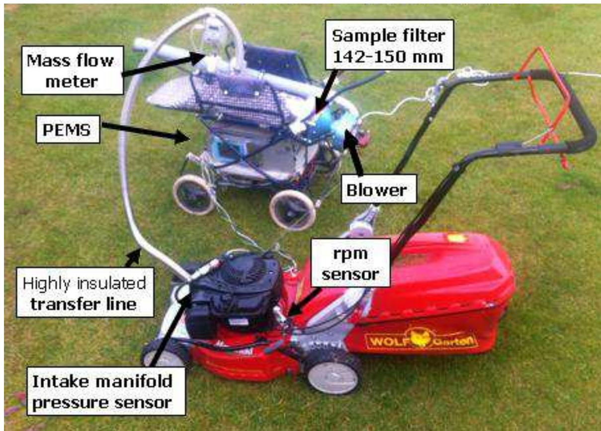
**Figure 1:** Off-board monitoring and sampling system [21]
