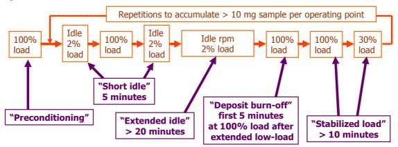
Raw exhaust was diluted at nominally 10:1 dilution ratio and sampled by a Hi-Vol sampler (EcoTech 3000) with a  $PM_{2.5}$  impactor operating at 67.8 m<sup>3</sup>/h rate. A second Hi-Vol sampler was used to provide filtered dilution air. Dilution ratio was verified by  $CO_2$  concentrations measurements. Samples of PM were collected on 20x25 cm fluorocarbon coated and quartz filters, with accumulations of ten to several hundreds of mg of PM per
