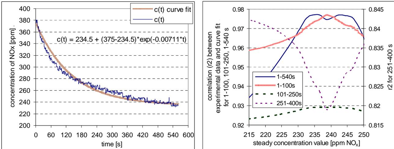
**Figure 7: Iterative regression of concentrations of NO<sub>x</sub> during idling of a Zetor 1505 tractor engine on heated rapeseed oil. Left: Experimental NO<sub>x</sub> concentration data and overall best fit. Right: Correlation between experimental data and fitted curve obtained using regression of multiple segments of the same series, as a function of steady value for concentration of NO<sub>x</sub>.**
