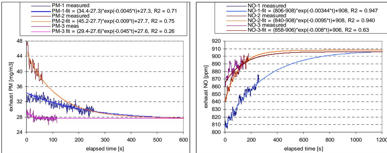
**Figure 5: Monte-Carlo iterative regression of multiple continuous subsets of experimental data with fitted curves and predicted steady values for operation at notch 8: concentrations of (a) PM and (b)  $NO_x$ .**
