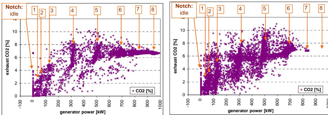
**Figure 3: Carbon dioxide (CO<sub>2</sub>) concentrations in exhaust gases of a diesel-electric locomotive as a function of generator power output: Aggregate data (left) over a high-load route run with a five-car train and (right) over a low-load route, mostly flat line traversed with a two-car train.**
