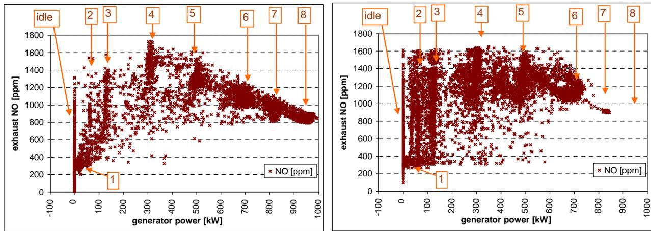
**Figure 2: Nitrogen oxides (NO<sub>x</sub>) concentrations in exhaust gases of a diesel-electric locomotive as a function of generator power output: Aggregate data (left) over a high-load route run with a five-car train and (right) over a low-load route, mostly flat line traversed with a two-car train.**
