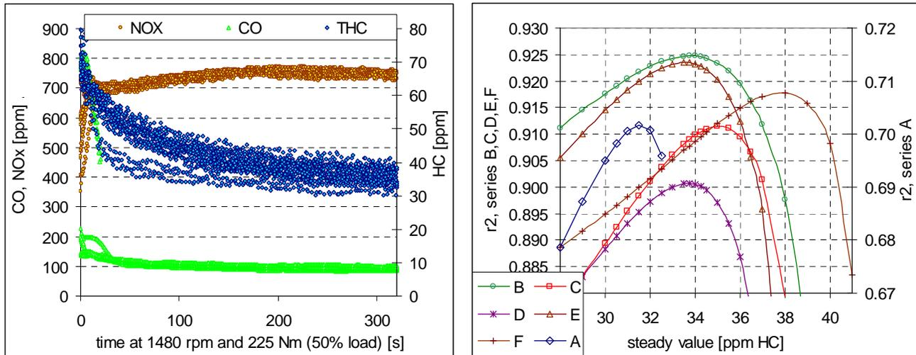
**Figure 9: Left: Concentrations of HC, CO and NO<sub>x</sub> during multiple occurrences of operation of a Zetor 1505 tractor engine on heated rapeseed oil at 1480 rpm and 225 Nm (50% load). Right: Correlation between measured HC concentrations and fitted curve obtained using regression of each data series, as a function of steady value for concentration of HC.**
