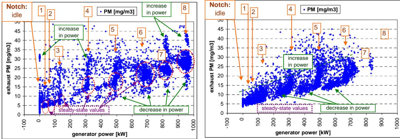
**Figure 1: Particulate matter mass (PM) concentrations in exhaust gases of a diesel-electric locomotive as a function of generator power output: Aggregate data (left) over a high-load route run with a five-car train and (right) over a low-load route, mostly flat line traversed with a two-car train.**
