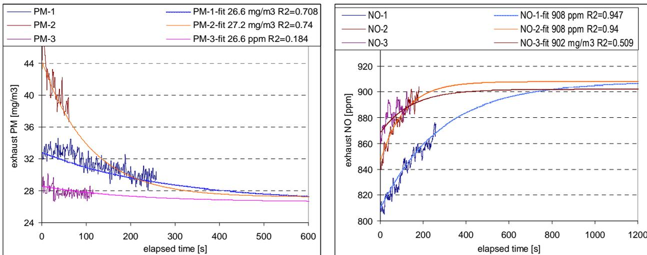
**Figure 6: Iterative regression of multiple continuous subsets of experimental data with fitted curves and predicted steady values for operation at notch 8: concentrations of (left) PM and (right) NO<sub>x</sub>. Regression was solved analytically for a user-supplied steady value and steady value yielding highest correlation between experimental and fitted data was selected.**
