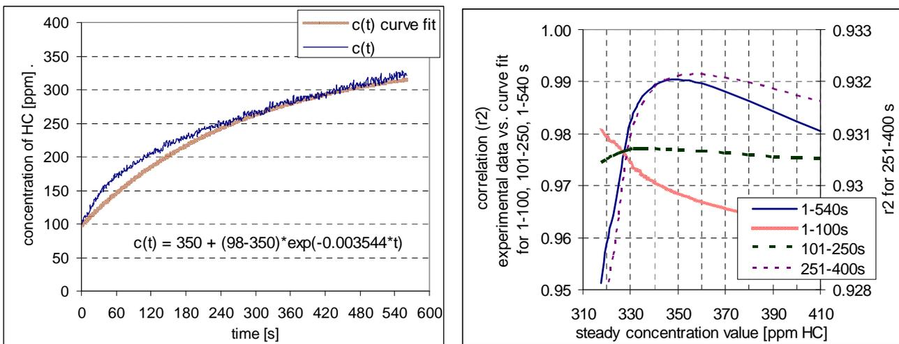
**Figure 8: Iterative regression of concentrations of HC during idling of a Zetor 1505 tractor engine on heated rapeseed oil. Left: Experimental HC concentration data and overall best fit. Right: Correlation between experimental data and fitted curve obtained using regression of multiple segments of the same series, as a function of steady value for concentration of HC.**
