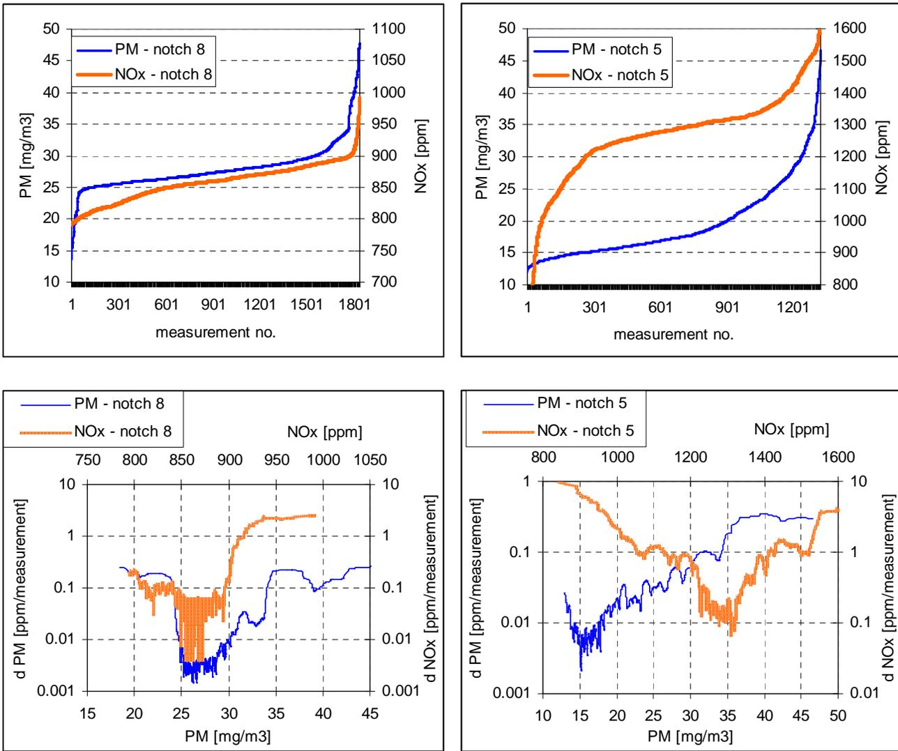
**Figure 4:** Top graphs show PM and NO<sub>x</sub> concentrations during all occurrences of operation of a diesel-electric locomotive (left) at notch 8 and (right) at notch 5, aggregated over all test runs, sorted by and plotted as a function of the measured concentration value. Bottom graphs show derivatives (rolling average of each 15 consecutive numerical values) of PM and NO<sub>x</sub> concentrations plotted in the upper graphs.
