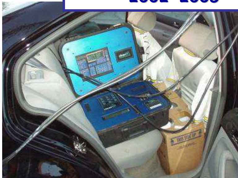
Commercially sold PEMS Montana system 2002-2005
