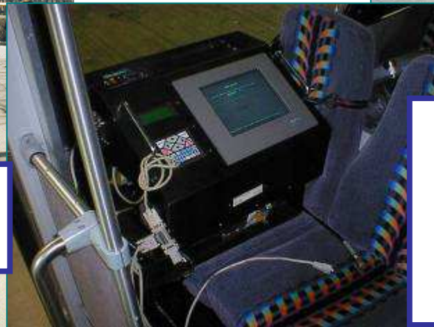
First commercially available PEMS - OEM-2100 Manufactured 1999-2002
