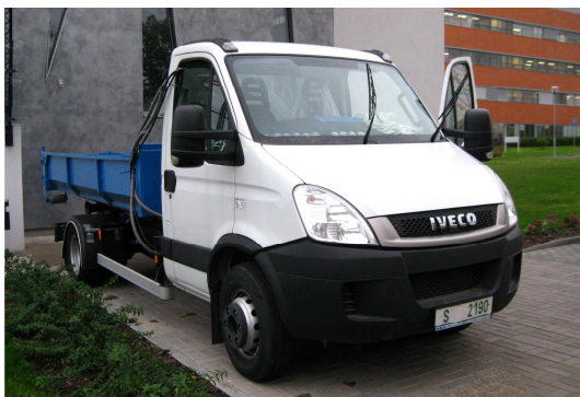
EURO 5 – DOC, DPF (particle filter), no SCR 2012 Iveco Daily, 3.0-liter Iveco engine
