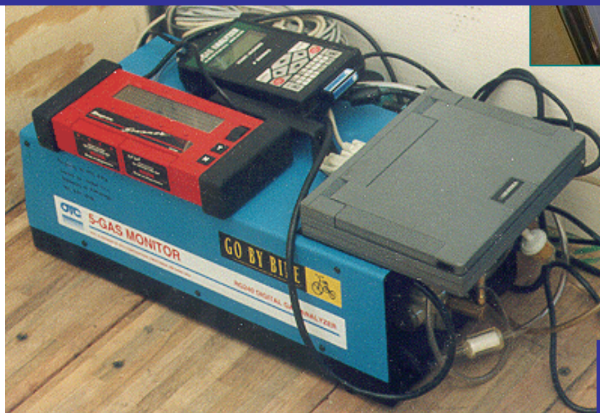
First PEMS used for CNG bus studies Pittsburgh, USA, 1996-1999
