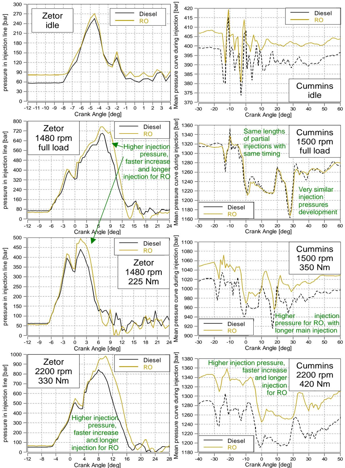
**Figure 3:** Comparison of pressure before injector on Zetor and Cummins for selected regimes
