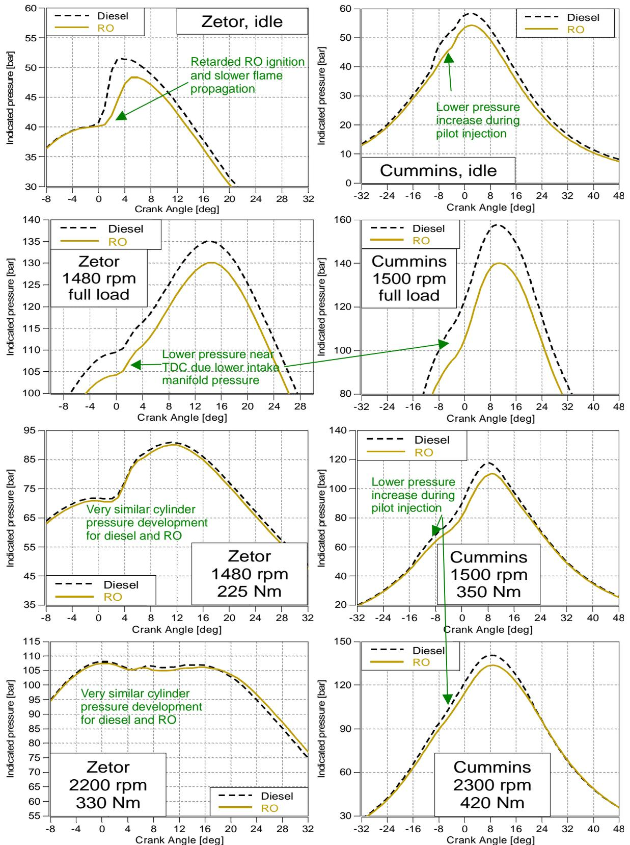
**Figure 4:** Comparison of indicated pressures on Zetor and Cummins for selected regimes
