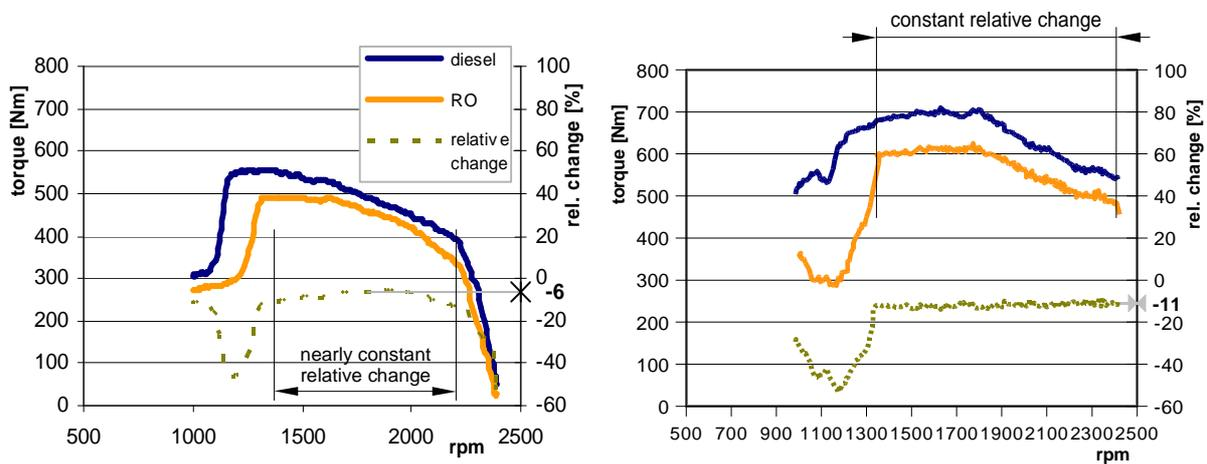
**Figure 1:** Comparison of torque curves for both engines (Zetor on left, Cummins on right) during operation on diesel and heated fuel-grade rapeseed oil
