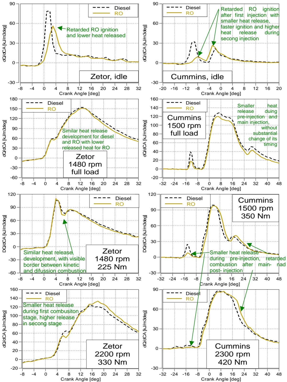
**Figure 5:** Comparison of released heat on Zetor and Cummins for selected regimes
