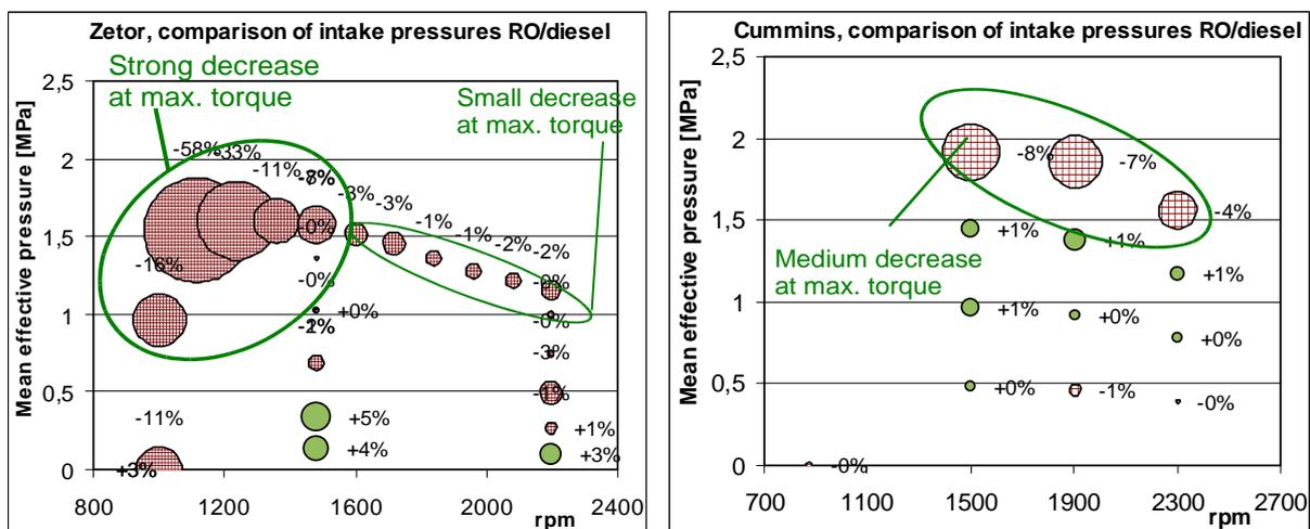
**Figure 2:** Intake manifold pressures comparison
