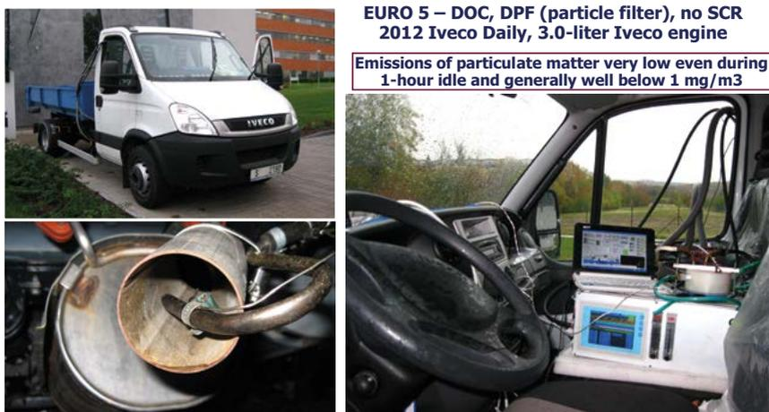
**Fig. 14: Vehicle #1, Iveco Daily Euro 5 with a diesel particle filter (DPF).**
