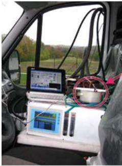
**Portable on-board exhaust emissions monitoring system (current version)**
