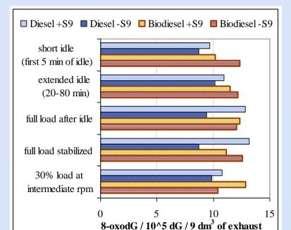
Fig. 3 DNA oxidative damage per volume of undiluted exhaust
