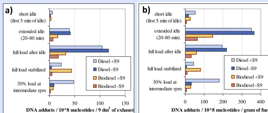
Fig. 2 DNA adduct levels per volume of undiluted exhaust (a) and gram of fuel (b)
