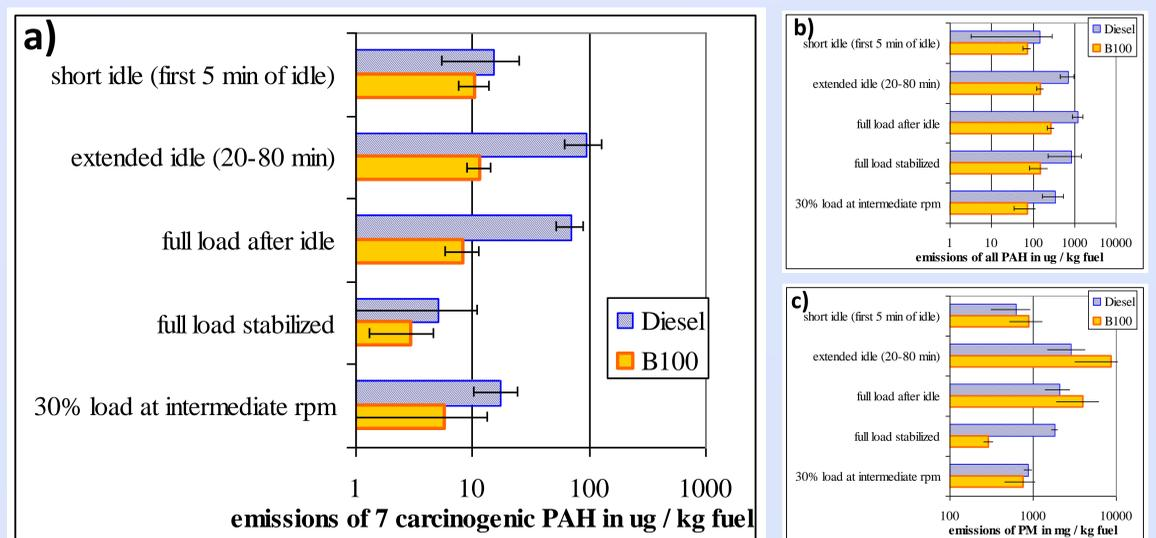
Fig 1 Comparison of fuel-specific emissions of a) cPAH, b) all PAH c) total PM mass
